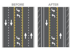
This five-lane to three-lane Road Diet removes lanes to allocate space for multipurpose use.
